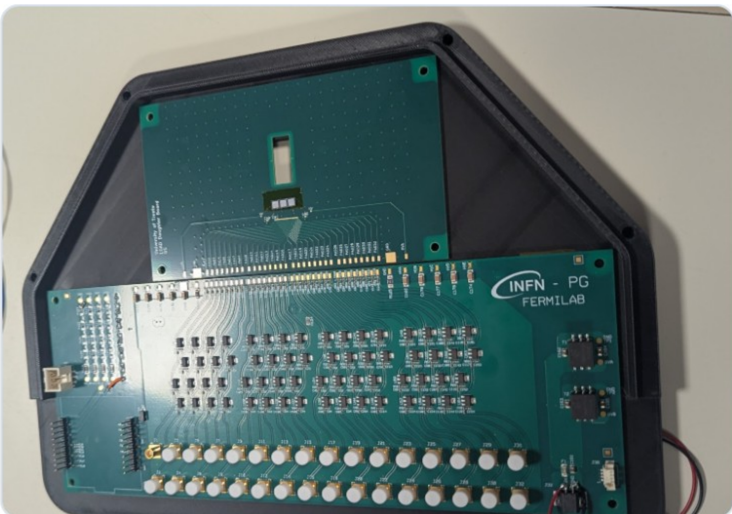
Full read-out chain: UnitN daughter board + INFN-PG / Fermilab 32-channel amplification board in the 3D-printed holder.
